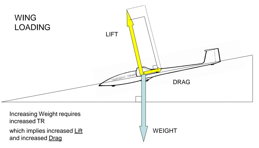
The lift required is referred to as the Wing Loading
